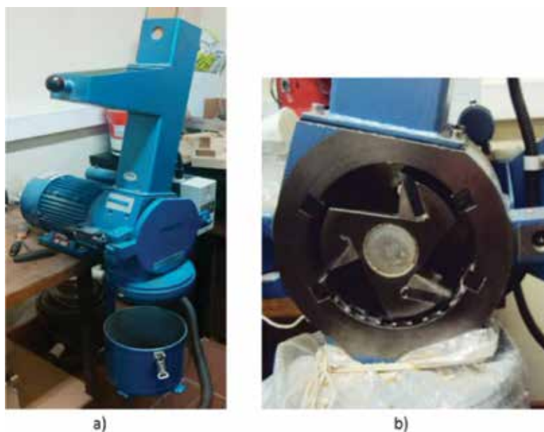
Figure 6. Cutting mill device: (a) general view and (b) cutting blade.
