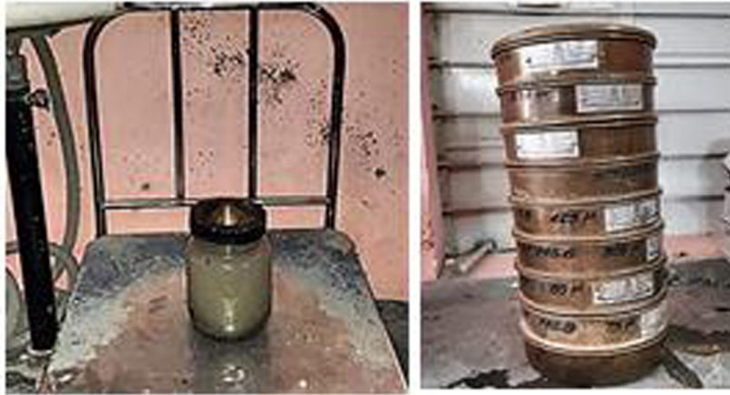
Fig. 3. Specific Gravity & Sieve Analysis of Fine Aggregate.
