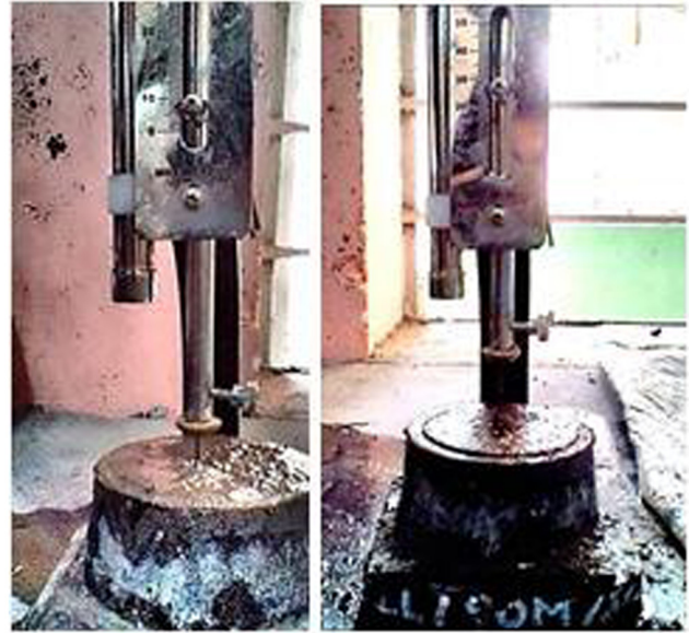
Fig. 2. Initial Setting & Final Setting Time.
