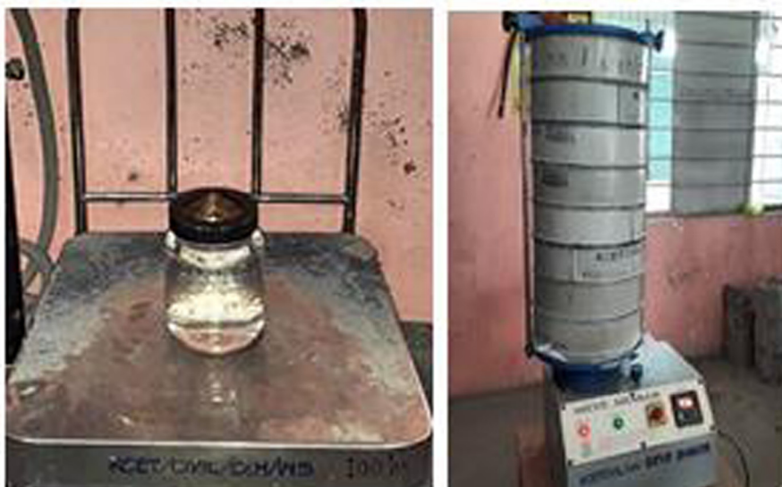
Fig. 4. Specific Gravity & Sieve Analysis of Coarse Aggregate.
