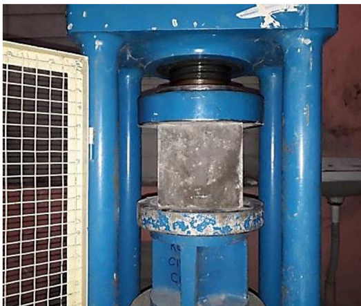
Fig. 5. Testing of Cubes.
