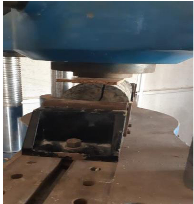
Fig. 6. Splitting Tensile test on cylinder.
