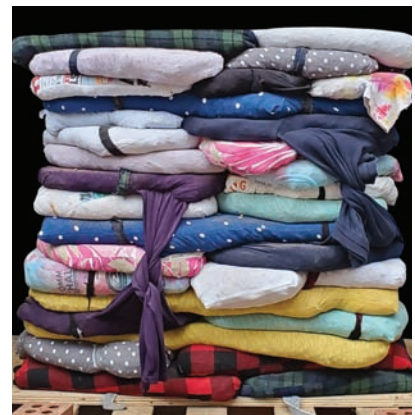
△ Figure 16. Pillow Earthbag wall prototype featuring an earth-infill with a sand additive. Recycled elastic waistbands tie down the barbed wire in between each layer, using bricks as weight.
