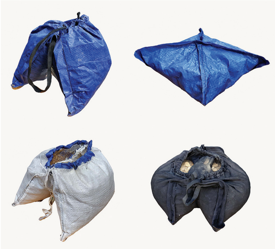
◀ Figure 18. 3D models of alternate earthbag geometries and materials through photogrammetry.
