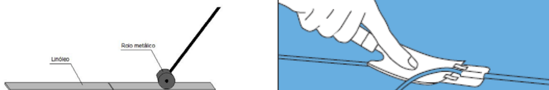
Figure 5 – Passage of a metal roller (left) and slider guide and spatula (right)
