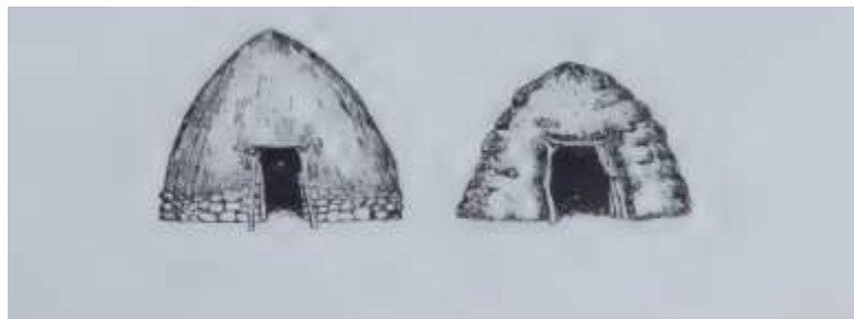
Figure 14: A figure showing the roof of poles leaning against a central framework, in the Susan Denyer classification ©Susan Denyer 1978.
