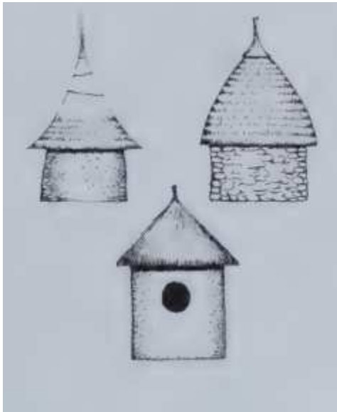
Figure 13: A figure showing the conical or trumpet-shaped thatched roof, in the Susan Denyer classification ©Susan Denyer 1978.
