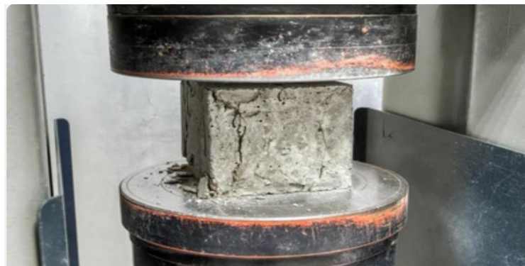
Figure 1: Crack pattern of the failed cube.
