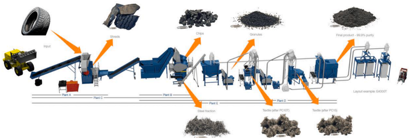
Fig. 5. Recycling process of waste rubber on a commercial scale (Recycling, 2022).
