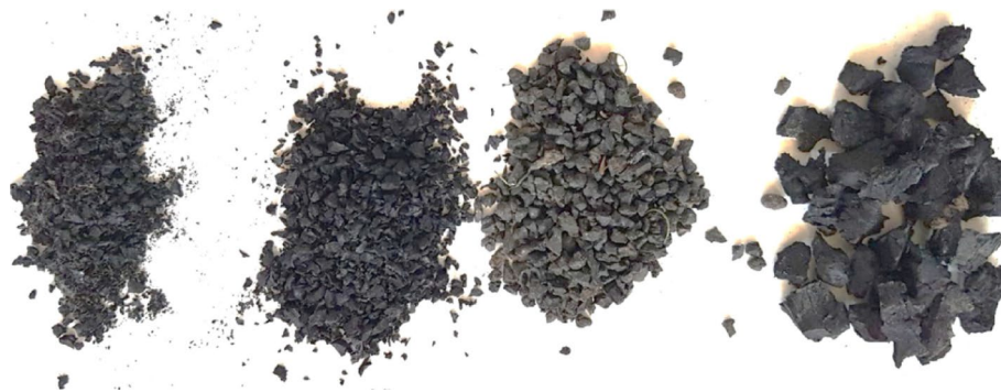
Fig. 2 Examples of recycled rubber aggregates with varying sizes [40]
