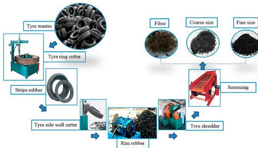
Fig. 1 Illustration of the approach for converting end-of-life waste tires into aggregates and fibers for construction materials [59]
