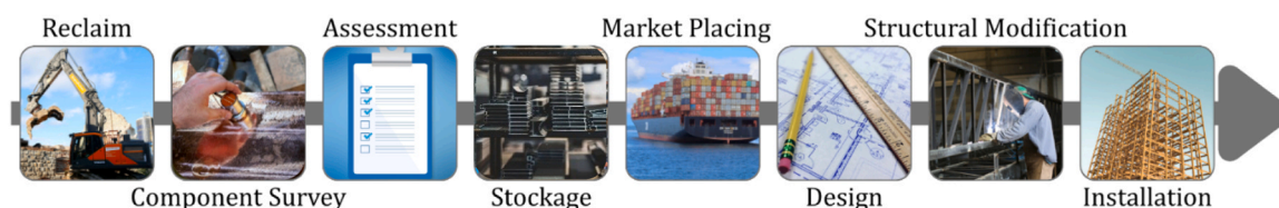
Fig. 6. Processes during reuse of reclaimed steel components – Variant 1.
