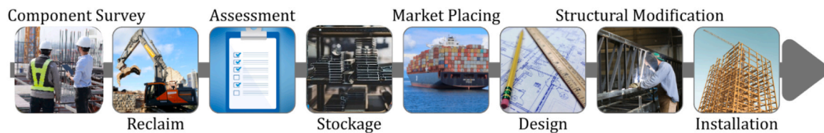
Fig. 7. Processes during reuse of reclaimed steel components – Variant 2.
