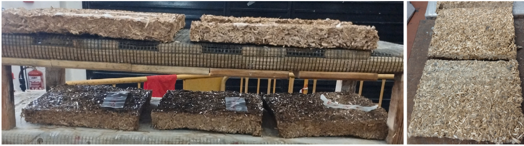
Fig. 2. Durability samples storage in laboratory conditions (right) and recycled samples (left).
