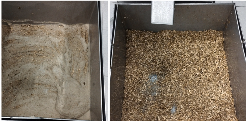
Fig. 3. Foam produced in the pulper by the recycled samples (left) and cleaned recycled raw material (right).
